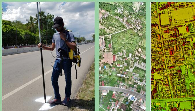
Performing a GNSS survey of ground control points (left). Their locations were included in image processing to improve deliverable geometry (right)
