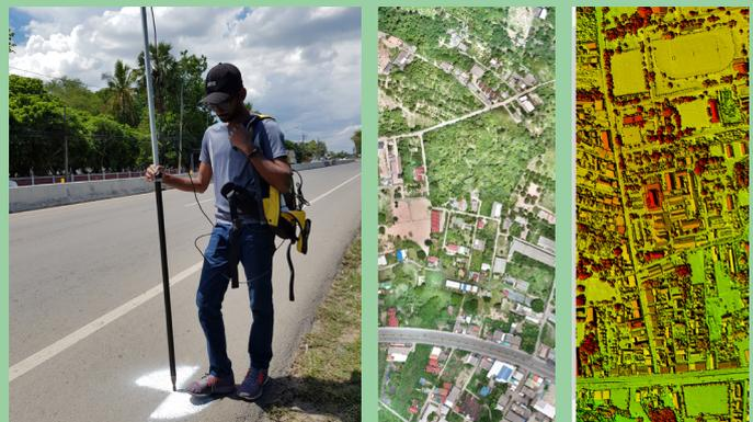
Performing a GNSS survey of ground control points (left). Their locations were included in image processing to improve deliverable geometry (right)
